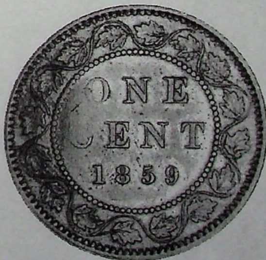
Figure 12. 1859 N9 Cent Showing a Large Area of Die Collapse at the Left
