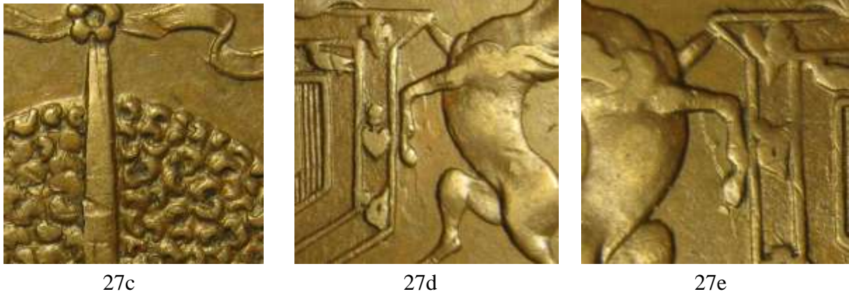
Fig. 27: Co. 7 a) obverse; b) reverse; c) pattern of wool resembling “25”; d) irregular incuse line possibly caused by extraneous matter on the punch; e) die clash on reverse showing head and foreleg of ram from the obverse. Author’s collection.
