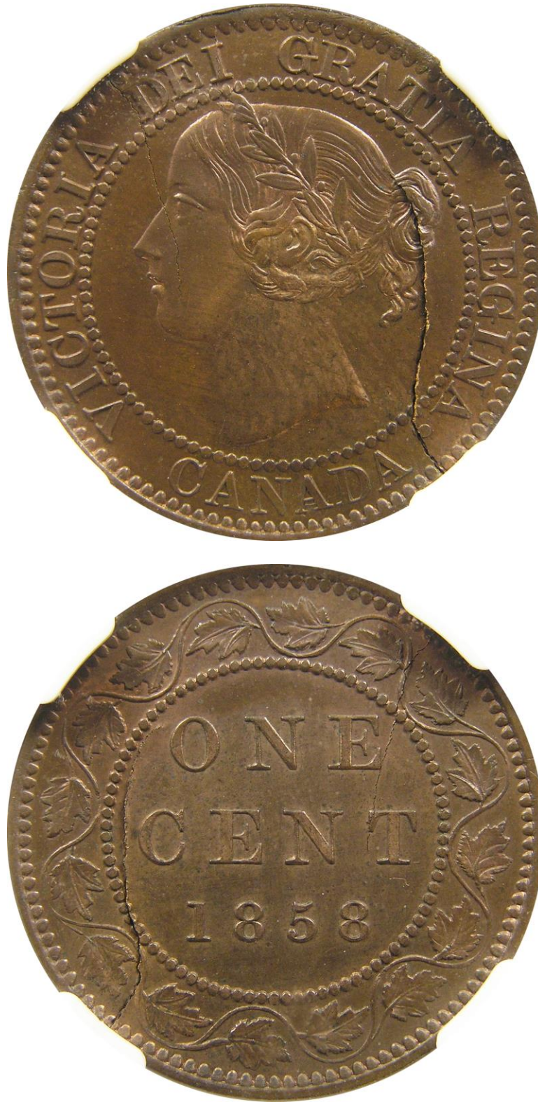
A nice example of a coin minted by Dies OB9/RC23 on a planchet cracked in two places; one starting left of the D in DEI and one near the dot in the legends. A grading service labeled this a mint state coin, but the die state, as indicated by the extent of the obverse die crack through the I in DEI, suggests the mint struck this coin as a specimen. (Photos by the author.)
