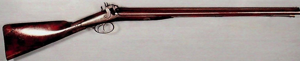
2181 Canadian Half Stock Percussion Three Barreled Gun , shotgun-rifle combination. 26 inch, 14 gauge side by side shotgun barrels and a .38 caliber rifled barrel above. Fixed front sight and an adjustable elevation fold down rear sight on barrel tang. Two back action locks marked T.J. BOYD behind the hammers. Platinum blow out plugs. Iron furniture elaborately engraved with floral patterns and hunting scenes on lock plates, trigger guard, barrel tang and butt plate. Iron ramrod pipes and a brass tipped wooden ramrod. Walnut stock with four iron plates screwed at a break in the wrist (this is an old repair). Overall length 43 inches. $1000
