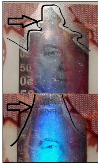
Image 5. Two different types of varnish design on the back of $50 Frontiers Series polymer notes—top is contoured around maple leaves and bottom is not contoured
