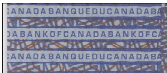
Image 2b – Magnified view of Micro text located as per Image 2a – English and French on alternating lines (Only four of twenty-one line shown)
