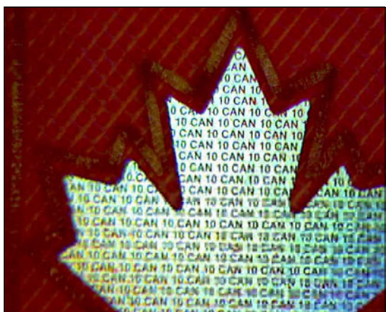
Image 9b – Magnified view of feature located as per Image 9a – repeating “10 CAN” text
