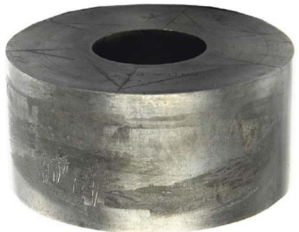
Figure 2. The die transfer roll produced from the vignette die plate of Figure 1. Image courtesy of Stack's 11/14/2007
