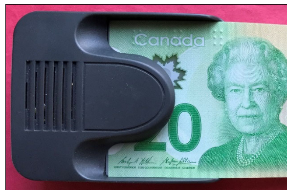
Image 2 — Canadian bank note reader by Brytech with $20 Frontier series note inserted to be read
