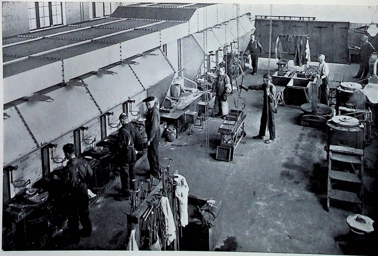
Chlorination Room, showing one side of bank of chlorination furnaces, with hoods and top of flue
